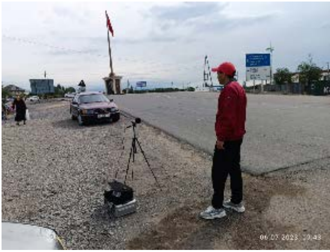
Photo 115. Lot 1. Balykchy, roundabout. Noise and vibration measurements. July
