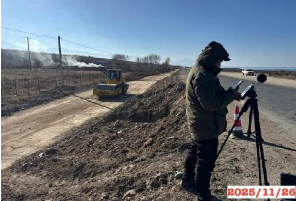
Figure 39: Noise and vibration measurements at the road site at km 160+120, Lot 1
