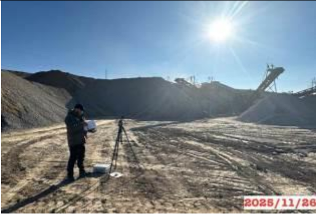
Photo 25. Noise and vibration measurements at the CSP production site, Lot 1, km 167+360
