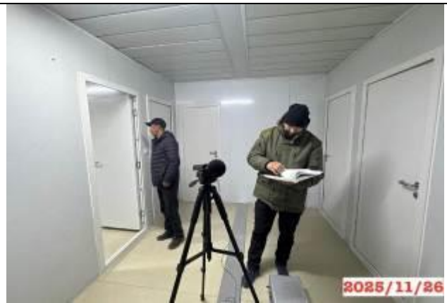
Photo 28. Noise and vibration measurements in the Consultant's office, The Ak-Terek Camp, km 152
