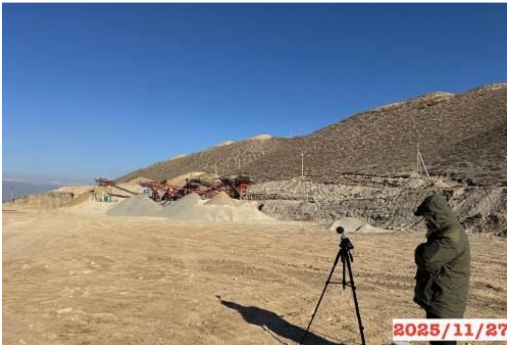
Figure 38: Noise and vibration measurements at the production site, CSP, Lot 2, km 202+220
