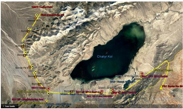
Figure 3: Location of noise, vibration, air and water quality monitoring sites
