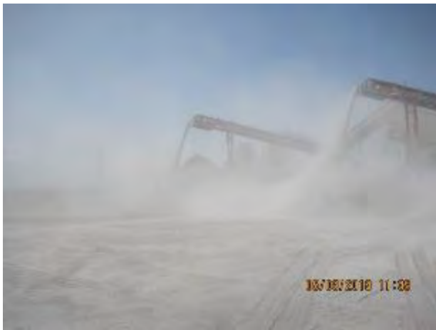
Figure 66 Operation of equipment without water sprinkling, with causing harm to the health of workers
