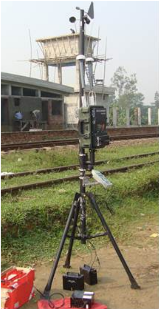
Figure 6: EPAS: Multi-probe scanner and data collection array in use on long term ADB-funded rail air quality and noise monitoring program
