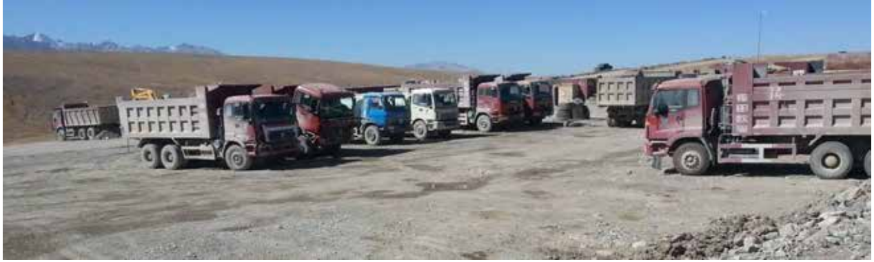
Figure 37: Overnight vehicle parking on rolled hardstanding
