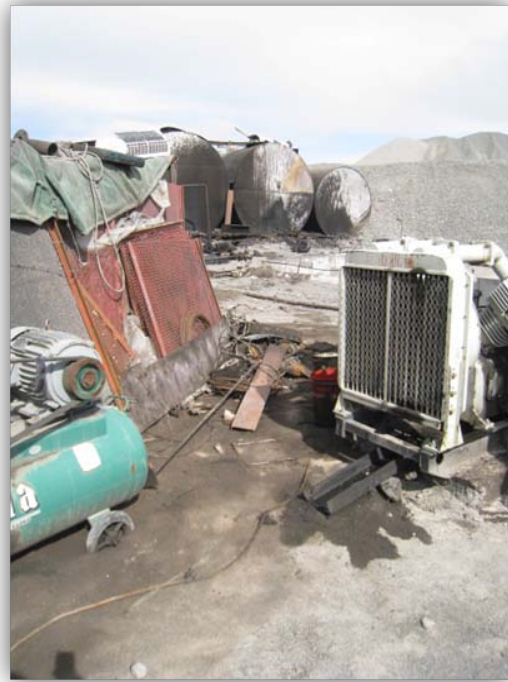
Picture 8. Team 2 ground: numerous and big spots of oil were found where there were not any protective coverage/cement coating
