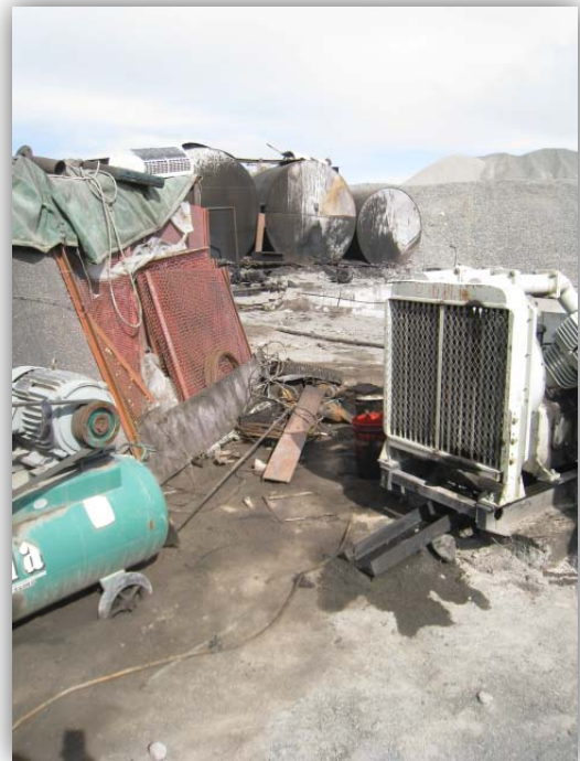
Picture 8. Team 2 ground: numerous and big spots of oil were found where there were not any protective coverage/cement coating
