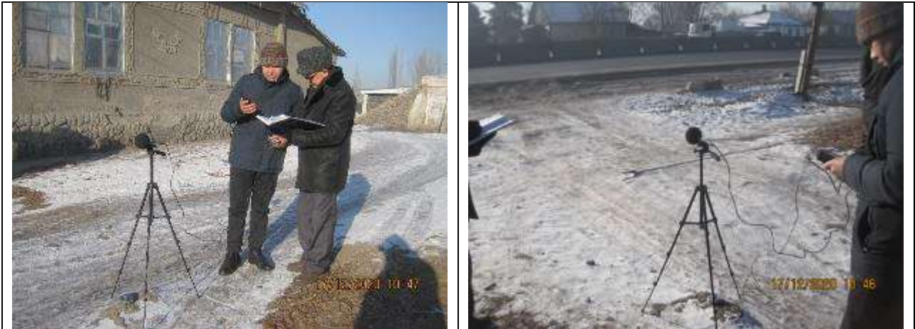
Figure 68 Noise level measurements in areas with a noise-reducing asphalt layer
