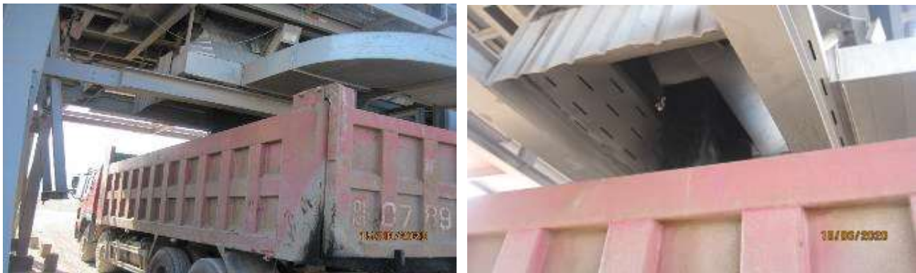
Figure 19 Loading asphalt mix in dump trucks
