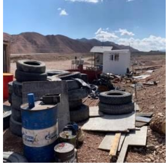
Photos 62. and Photo 63. The conditions of storage and keeping of materials and production waste do not comply with environmental requirements.
