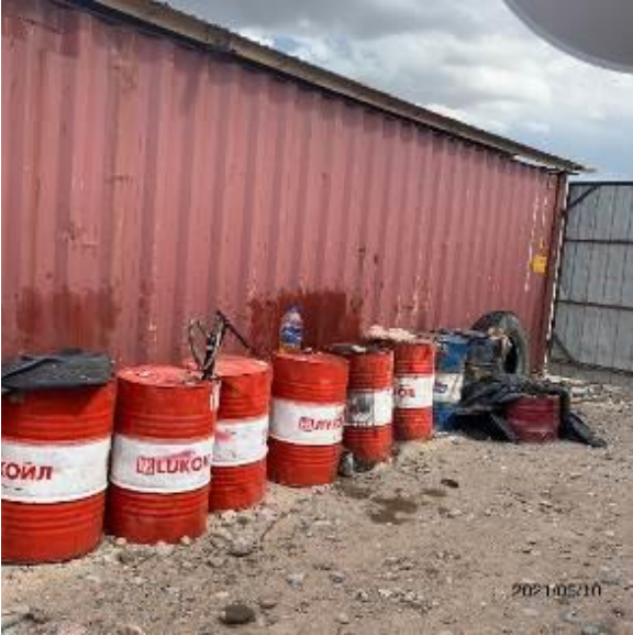
Photo 74. Lot 2. Storage conditions for fuels do not meet environmental requirements.
