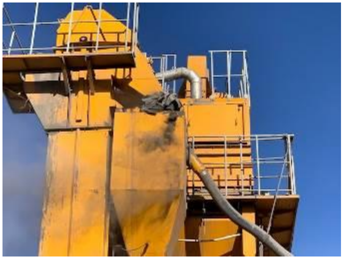
Photo 63 and 64. Lot 2. Emissions from the damaged sections on the connection hoses.
