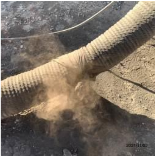
Photo 63 and 64. Lot 2. Emissions from the damaged sections on the connection hoses.
