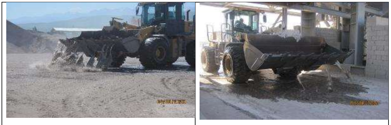
Figure 60 Watering of the production site with flushing water.
