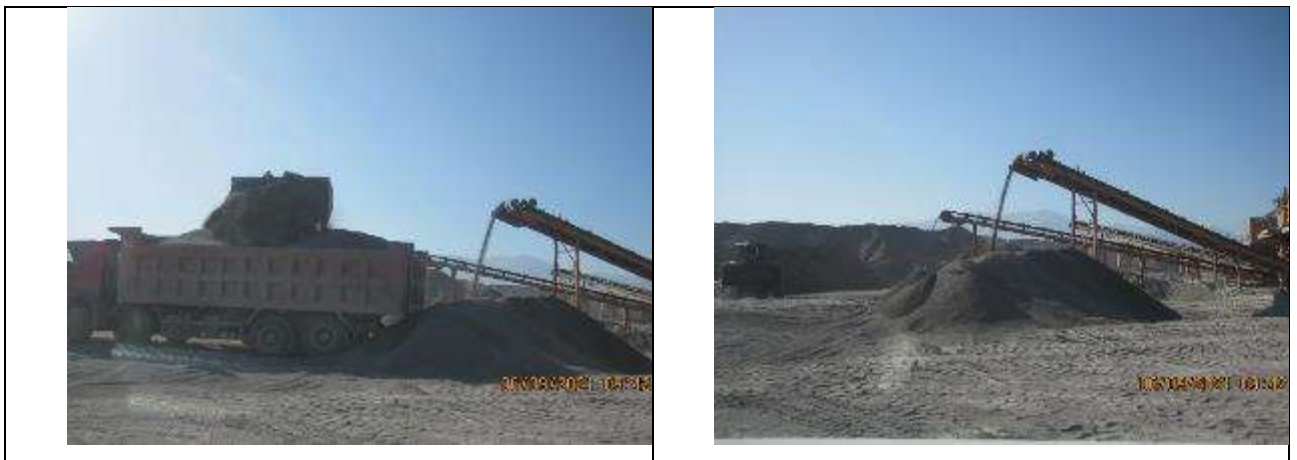
Figure 55 Operation of the stone crushing plant with moistened raw materials.
