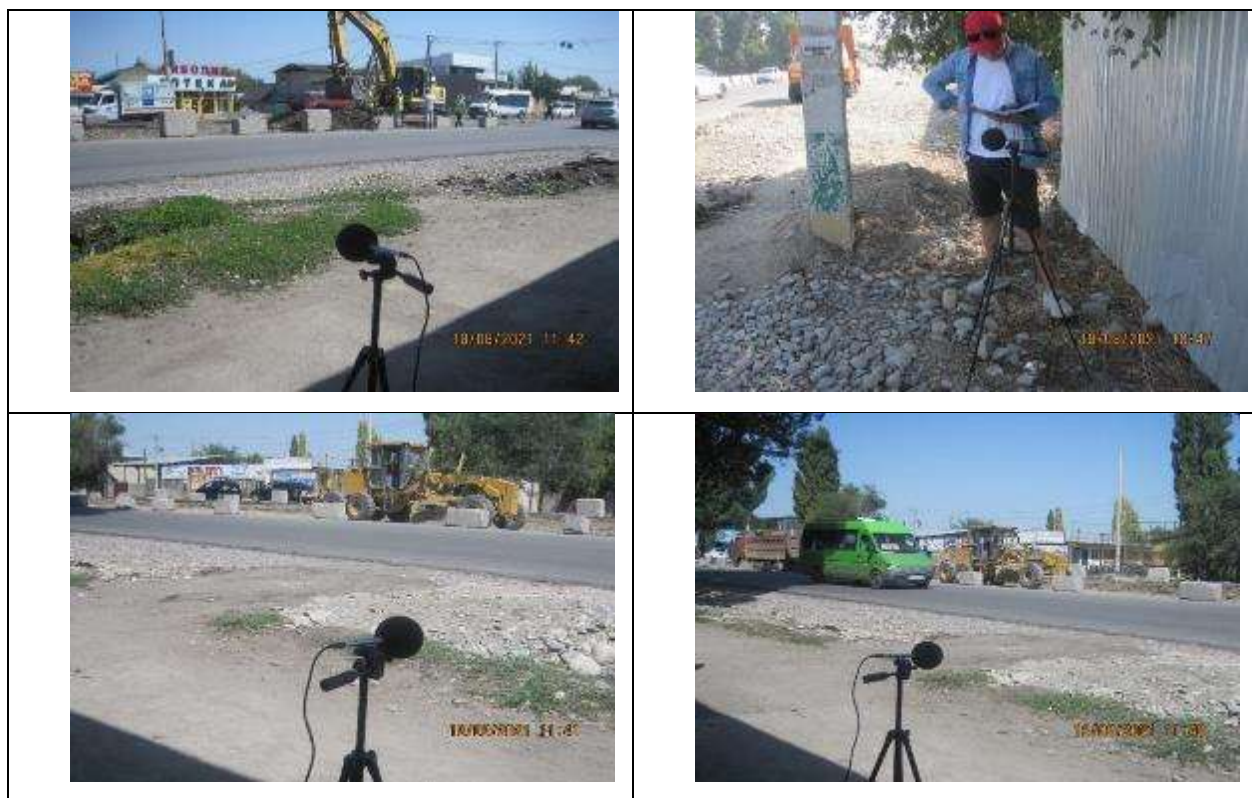
Figure 80 Conducting noise and vibration monitoring.
