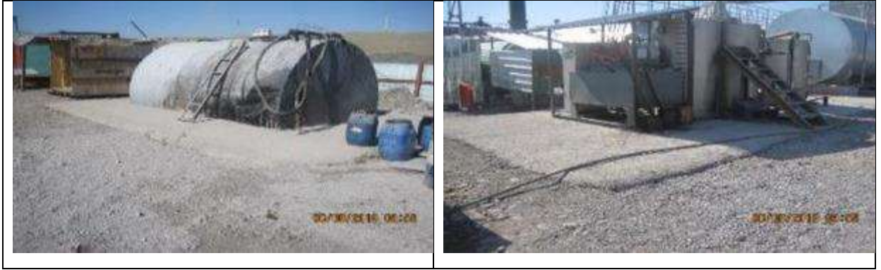
Figure 53 Impermeable protective coating around chemical containers.
