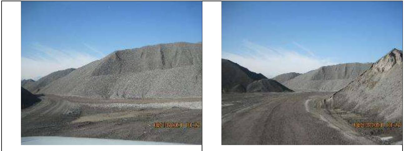
Figure 56 Prepared gravel material for the production of concrete and asphalt.
