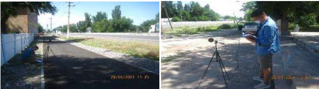
Figure 68 Noise level measurements in areas with a noise-reducing asphalt layer
