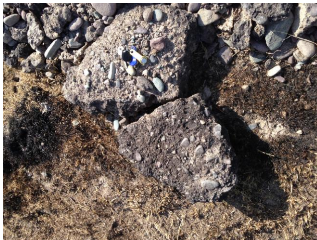
Figure 21. Close up of size of larger waste asphalt pieces; approximately 10cm x 5cm, which is crushed to a much smaller size after several bulldozer passes
