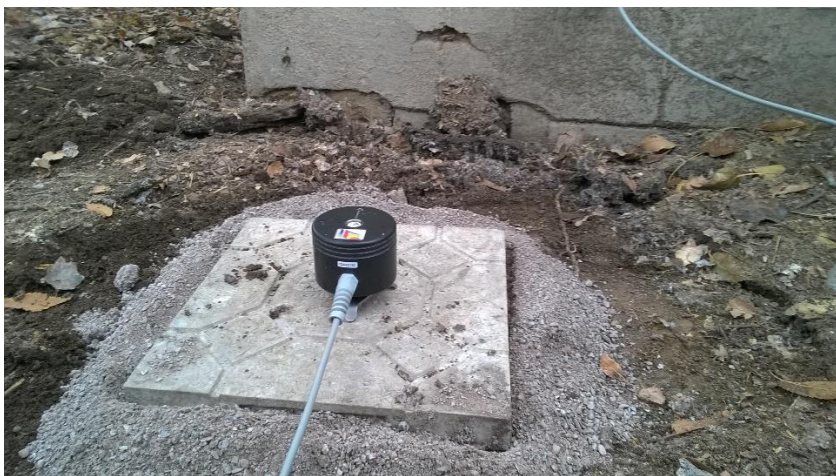
Figure 2. Location of Geophone on Slab adjacent to Foundation
